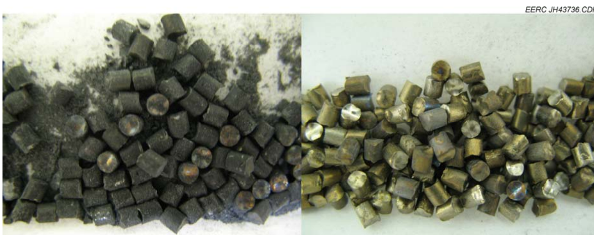
Figure 11. Close-up of the steel shot used in the methanol vaporizer showing deposits formed from carbon and potassium. The left picture is from the vaporizer testing the MILS methanol, and the right picture is from tests with commercial methanol.
