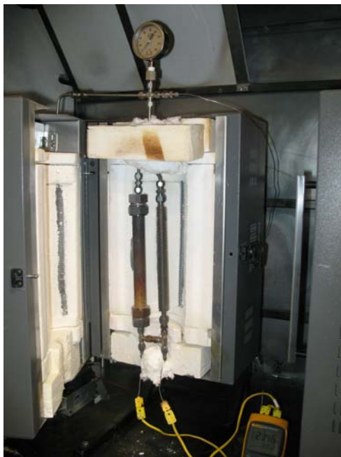
Figure 4: Image of test bench furnace with reactor (left) and fin-tube vaporizer (right).
