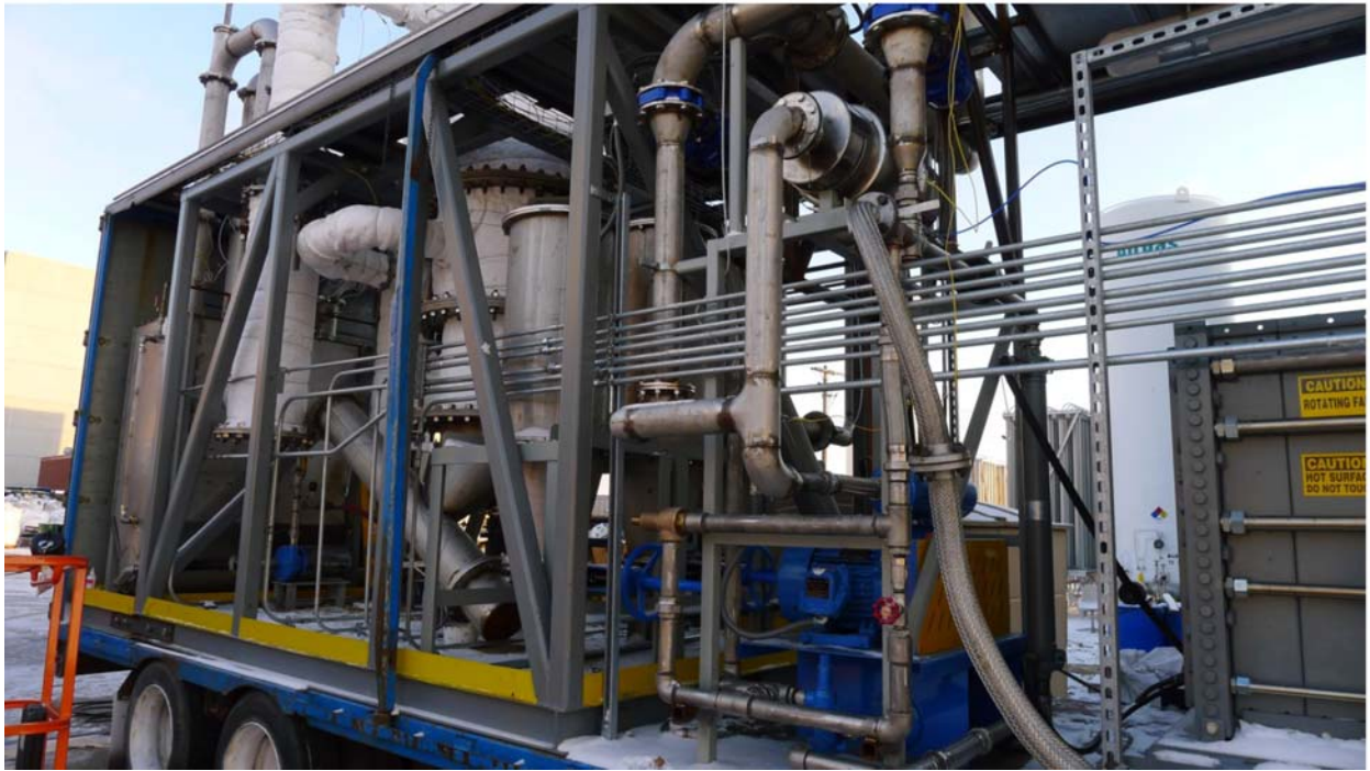
Figure 4. The MILS gasifier and gas-cleanup system.
