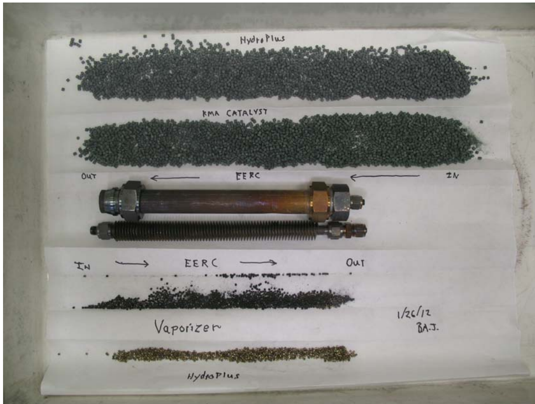
Figure 8: Image of the contents of the reactors used to reform HydroPlus (top) and EERC BioMethanol fuel (second from top) and steel shot from vaporizers for EERC BioMethanol fuel (second from bottom) and HydroPlus (bottom).
