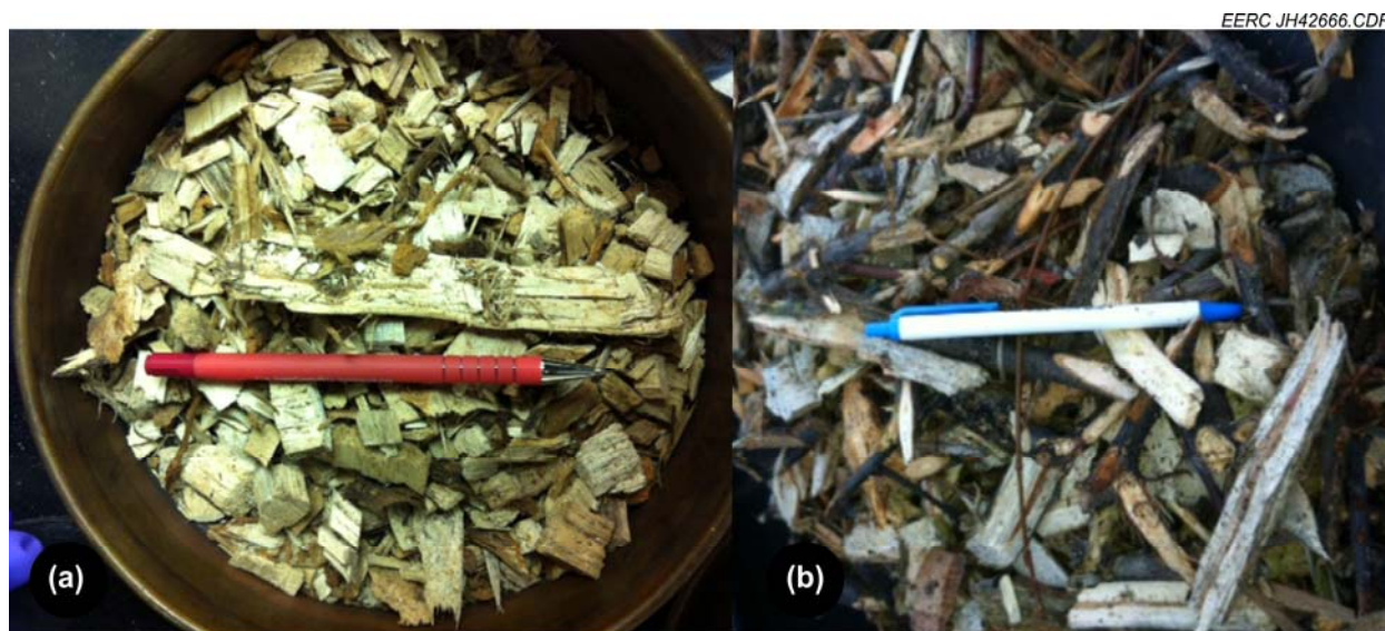
Figure 6. Biomass used in the experiments: a) chipped green poplar wood waste and b) city wood waste, primarily chipped ash.
